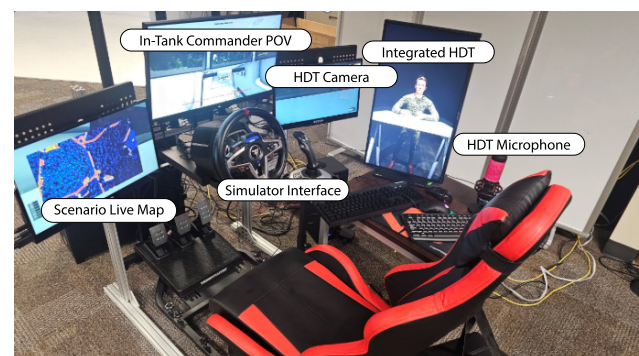
Figure 1: Annotated photo showing the system setup.
